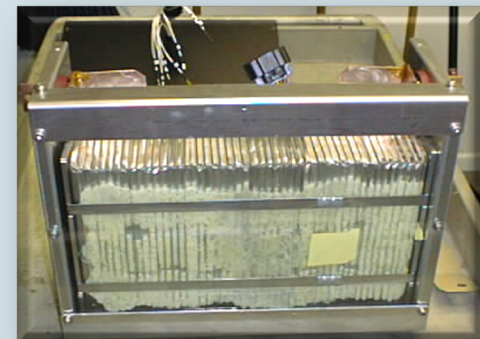
16 Module Altairnano Battery Pack 20kWh capacity
