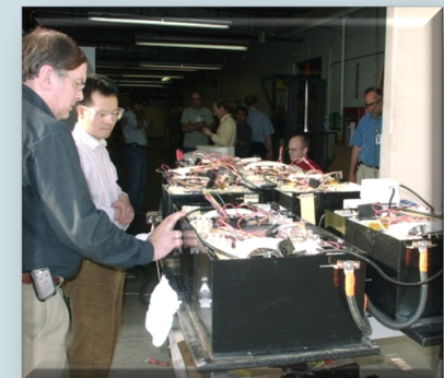
Altairnano Battery Pack 35kWh capacity
