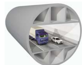
Possible Bored Tunnel (Viaduct Project Team Simulation)
