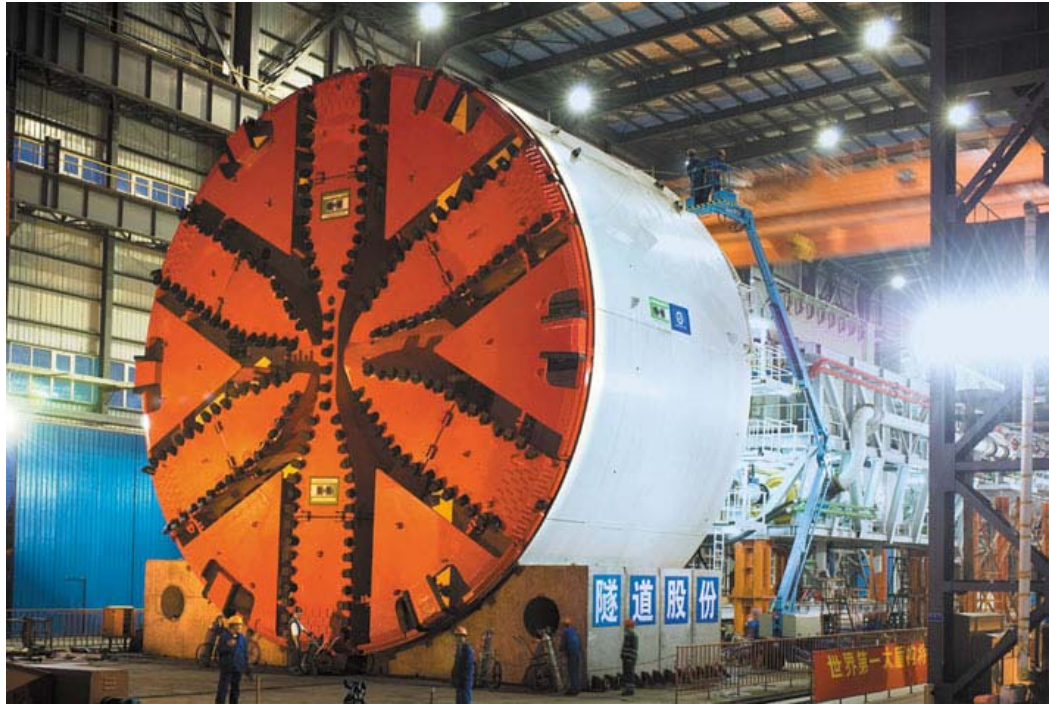
Figure 4: 51-ft Diameter Earth Pressure Balance Tunnel Boring Machine.
