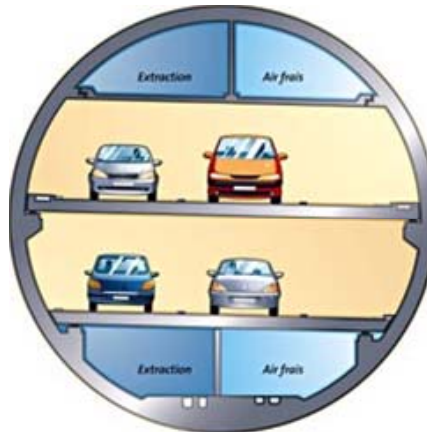
Figure 5: Typical two lane stacked tunnel section, A86 Paris.
