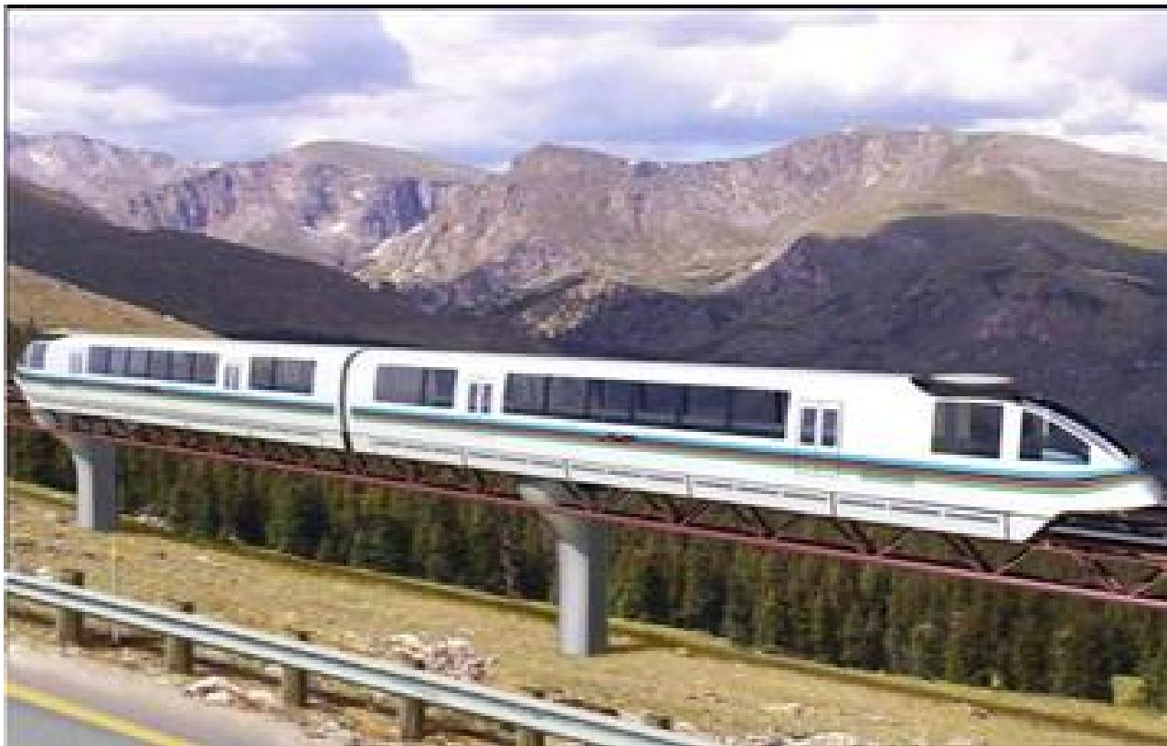
**Colorado 200 (FTA Study of CHSST Upgraded to 120 mph 10% grade [undegraded] for use in USA)**
